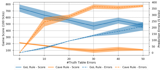
Fig. 2. Number of truth table errors ( \pm sd) plotted against game score after 100 ticks (solid lines) and against the number of prediction errors after 5 ticks (dashed lines). Results using the Game of Life update rule are depicted in blue, while orange corresponds to the Cave Generator update rule.
